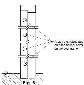
6. Attach the hole plates onto the anchors holes on the door frame and firmly press until completely flush on the door frame surface. (the hole plates have been provided together with the door).
