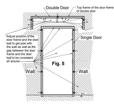
5. Insert u-washers and turn the bolts but not completely tight yet. Then close the door leaf again to check and adjust position of the door frame and door leaf to get plan with the wall as well as the gap between the door frame and the door leaf to be consistent all around.
