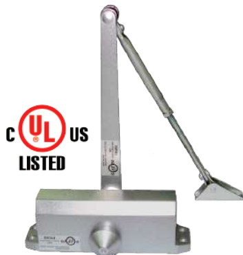
c UL US LISTED Swinging Fire Door Closer, Surface Mounted, Non-Hold Open, Regular Arm, 180°, 60-85 kgs, 3-Hour Fire Rating, UL 10C
