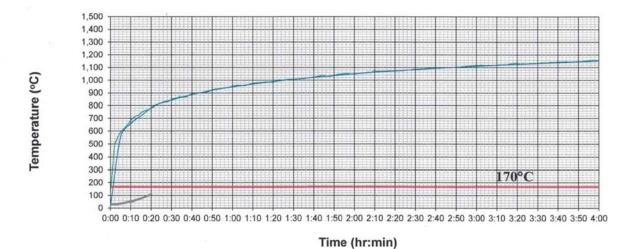
—Average Furnace Temperature —BS 476 —Average Specimen Temperature —Critical Temperature
