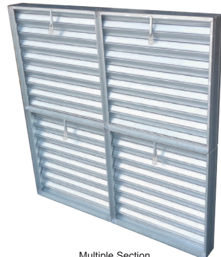
Multiple Section (4 units of single section connected together), In Airstream, automatically fully close when temperature reaches 165°F (74°C) to prevent fire flow through
