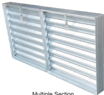
Multiple Section (2 units of single section connected together), In Airstream, automatically fully close when temperature reaches 165°F (74°C) to prevent fire flow through
