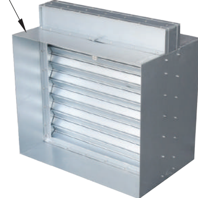
Single Section (with damper sleeve), Out of Airstream, automatically fully close when temperature reaches 165°F (74°C) to prevent fire flow through
